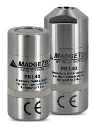
The 1/8" NPT pressure port featured on the device allows for compatibility with a variety of fittings and adapters. This is ideal for calibration purposes, as well as connecting the data logger to measure process pressure systems.
